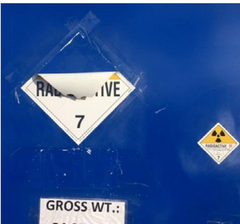
**Is placard durability and visibility during transport important?** Should both the shipper and carrier be responsible to meet the placard requirements in 49 CFR 172 Subpart F? Yes to both! 49 CFR 172.516(c) states placards must be securely attached and carriers must maintain placards. Also, 172.519(a) requires the placard to be able to survive normal conditions of transport.
