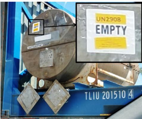
**This is interesting use of the white background space required on the Empty label!?! Seems very efficient, but is this compliant with the Empty label specifications in 49 CFR 172.450? Hopefully you answered "no" with yellow colored tape added.**
